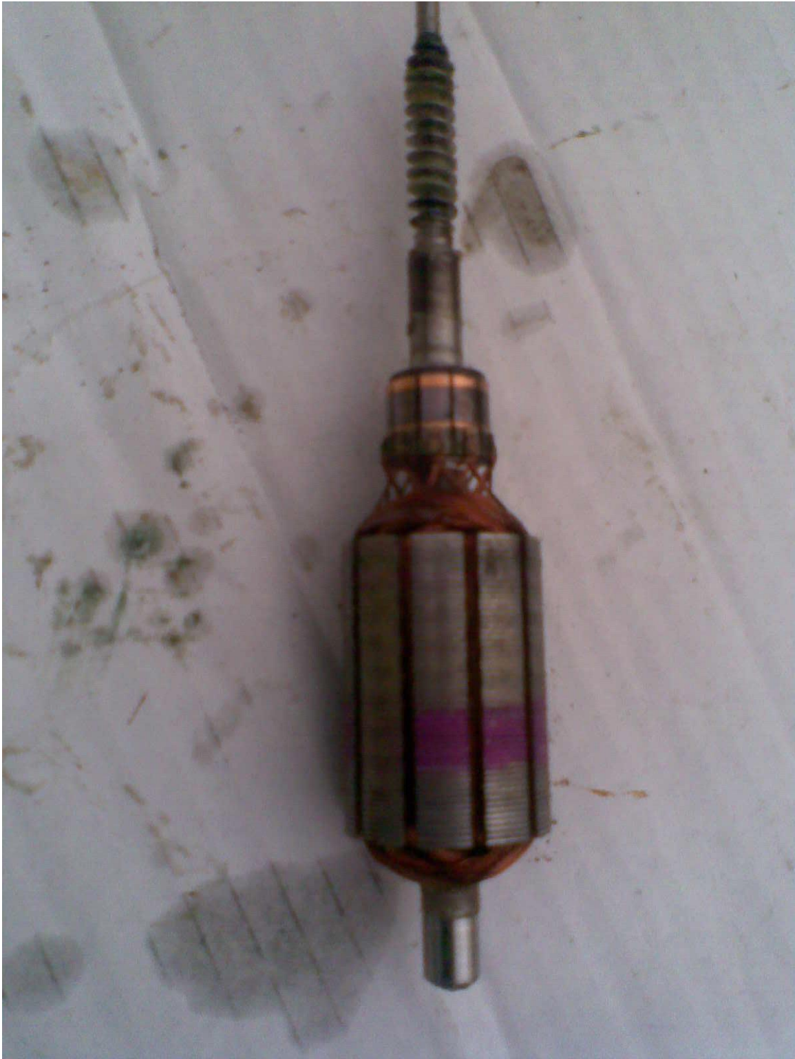
Photo Above - Rotor Before Cleaning
